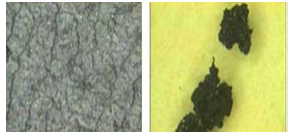
Fig.3 Wear pattern and particle size of normal sample
