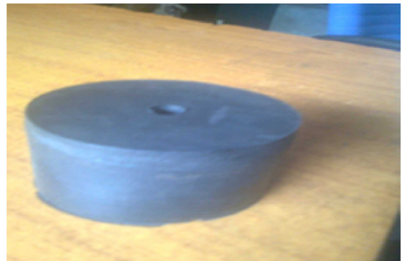
Fig.2 Model of a base isolator
