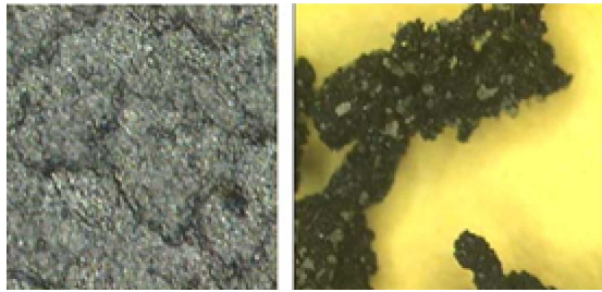
Fig.4 Wear Pattern and particle size of oil swollen samples
